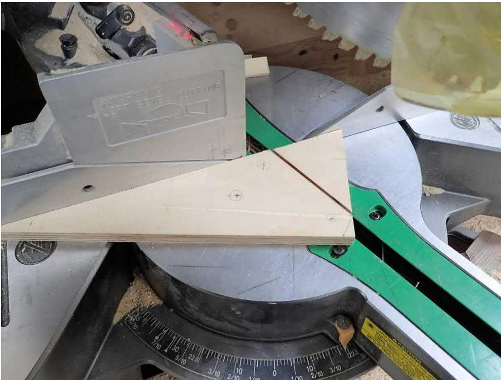
These angle cuts need not be overly precise, since they are at the top of the jig and don't have any bearing on the accuracy.
