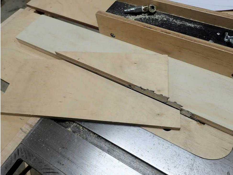
I cut the other angle at the miter saw, setting the saw to 22 degrees past 90:
