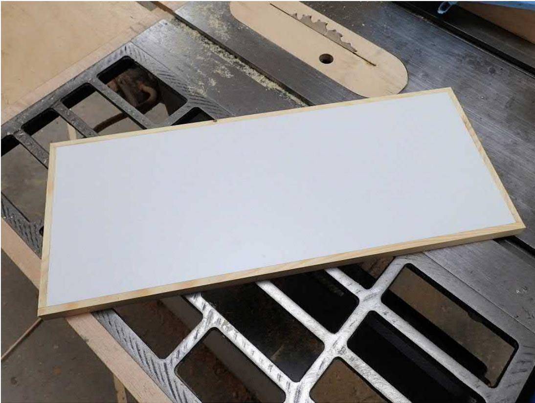
The strips that hold the stone in place and act as stops for the jig were added next:
