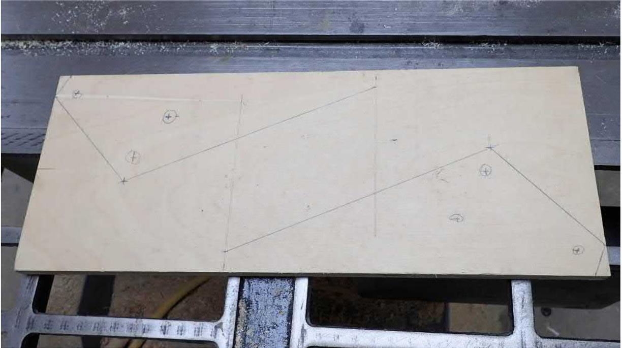
To cut the long angle, I used double sided tape to attach it to a straight board. I lined the edge up with the line drawn on the plywood, then cut it on the table saw:
