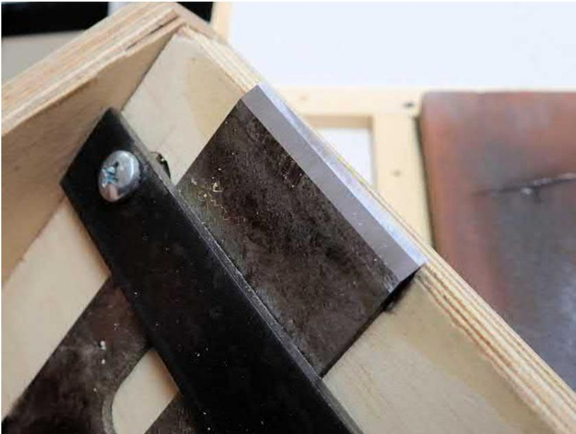
The stone I'm using has a coarse grit on one side (90 grit) and I use that to grind the primary angle. The other side is fine (600 grit) and I hone the secondary angle with it. Normally, that's as far as I'll go, since I've found that sufficient for most cutting operations.
