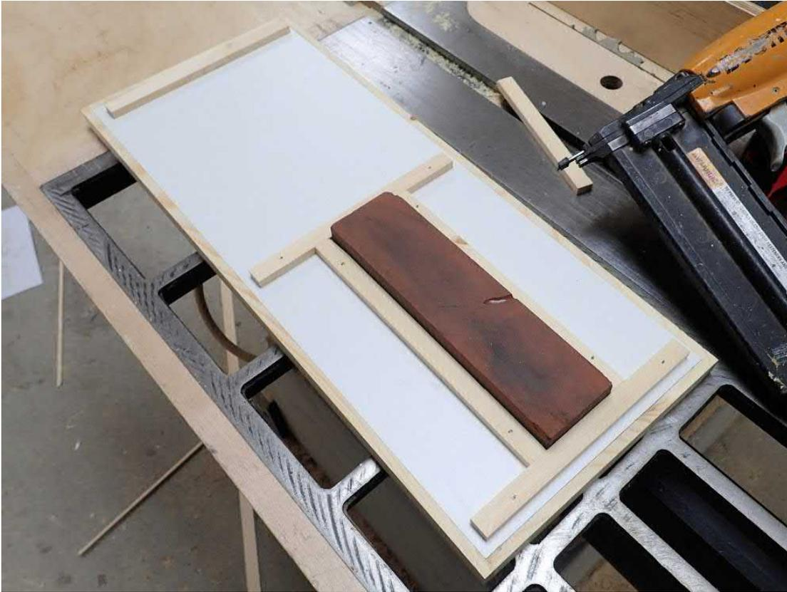
Stones shorter than 8" can be used, but the back stop strip should be move forward to keep the chisel / plane from slipping off the stone.
